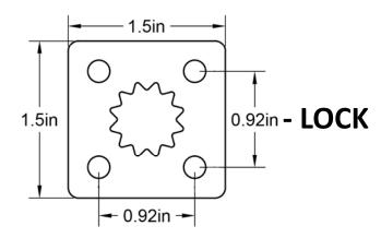
Side view of Lock unit not shown: Overall thickness of Lock unit is 3/8"
